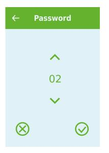
The service settings require a password because certain knowledge is necessary in order to change these settings. An incorrect setting may result in the unit not working properly.
